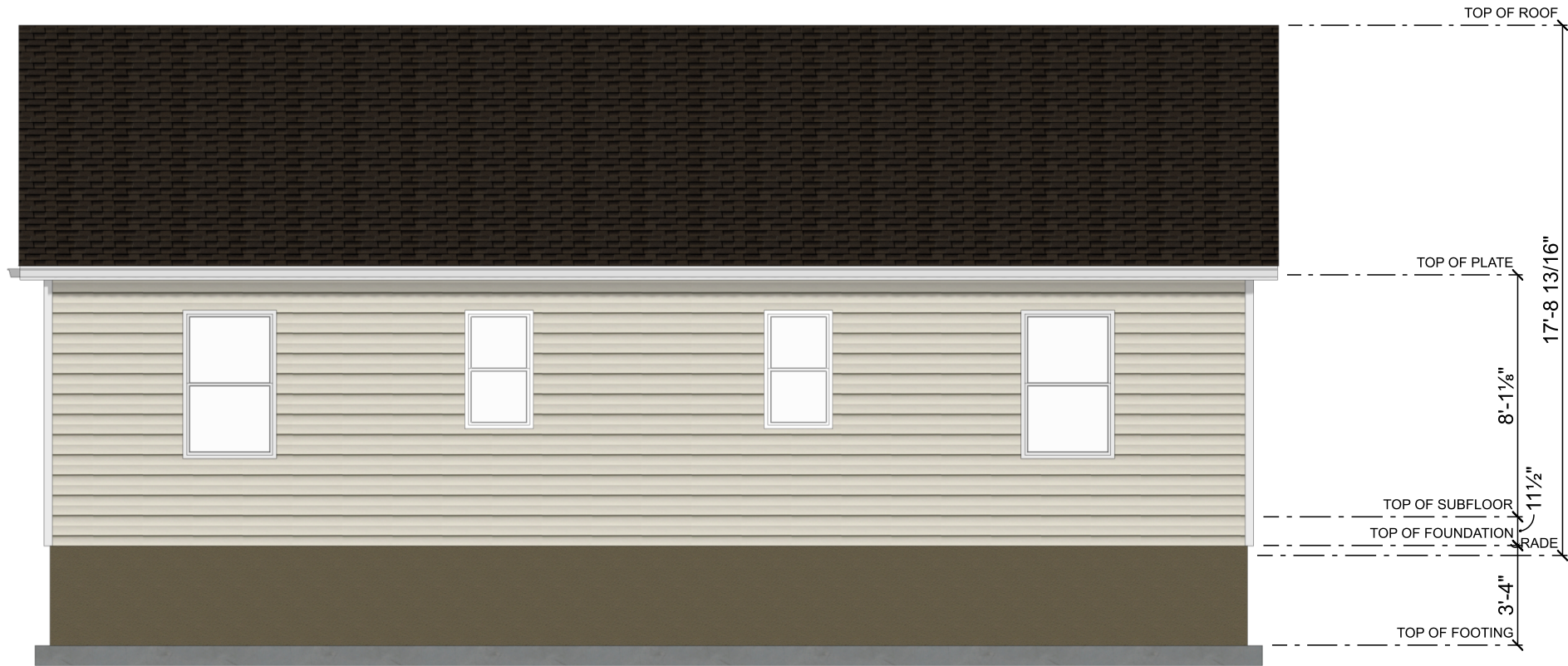
REAR ELEVATION SCALE: 3/16" = 1'-0"
